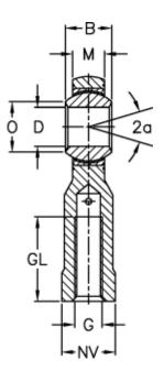
$\begin{array}{lll} A & = 42 \\ a \text{ (degrees)} & = 15 \\ B & = 21 \\ D & = 16 \\ Dynamic load C \text{ (kN)} = 52.5 \\ F & = 64 \\ G & = M16x1,5 \\ GL & = 28 \\ \end{array}$
